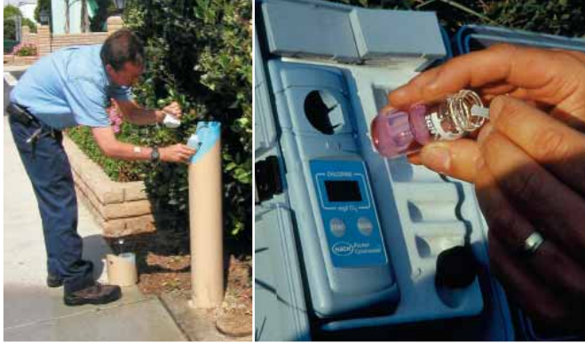
Figure 6.1 Manual Water Quality Sampling and Field Testing
